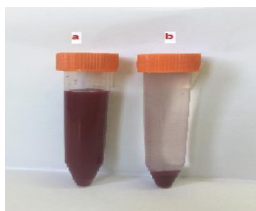
Figure 4. Adsorption of disperse dye with optimum dose of adsorbent, (a) starting solution of red disperse dye, (b) treated by hydroxyapatite.
