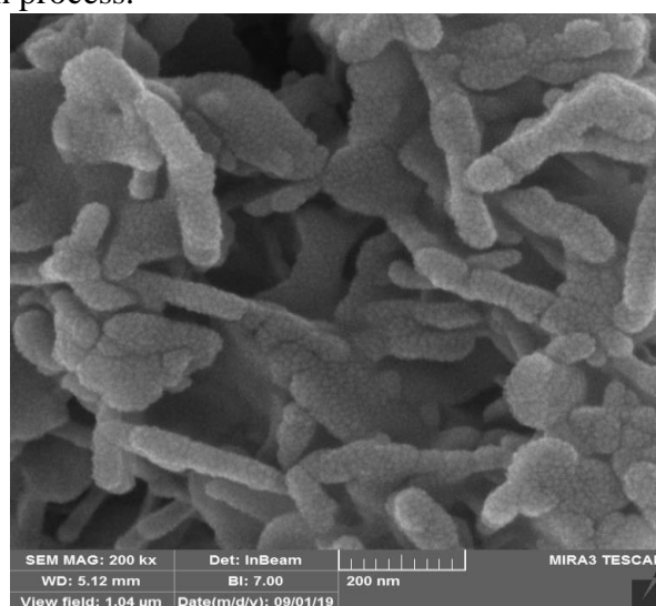
Figure 7. FESEM image of powder prepared by fuel ratio of 0.13 and pH: 7.0.
