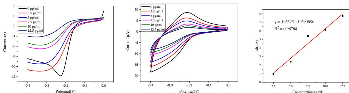
Figure 2: (a) CV tests, (b) SWV of PSA detection of labeled electrode by methylene blue in PBS, and (c) calibration curve of SWV
