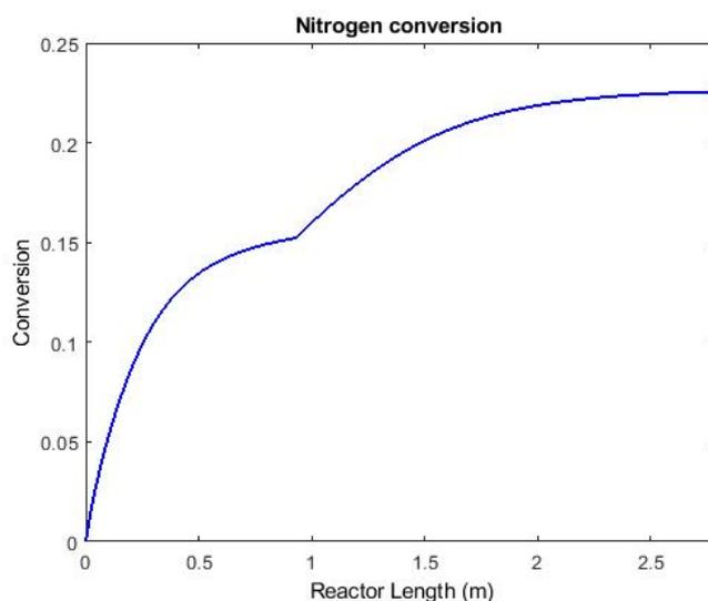
**Fig. 3 Nitrogen conversion along reactor**
