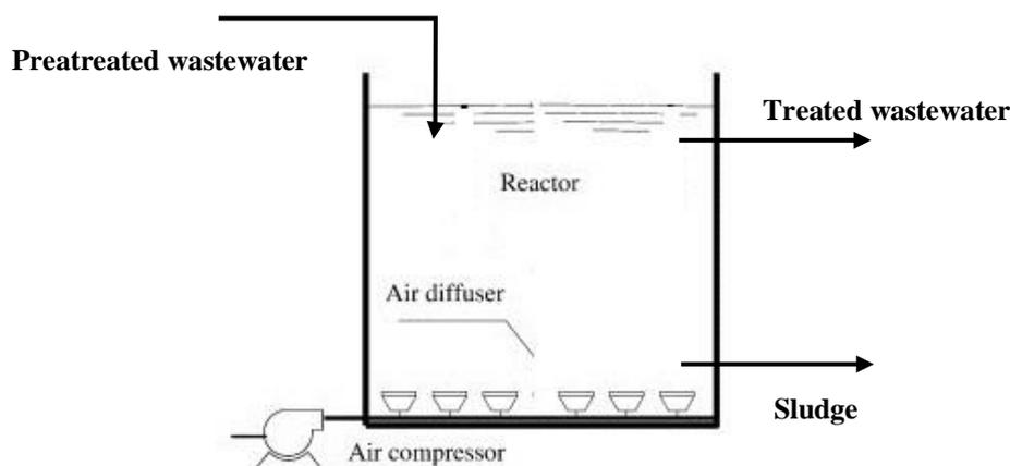
Fig. 1. Schematic structure of sequencing batch reactor (SBR).
