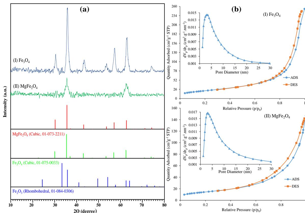
Figure 1. a) XRD patterns, b) Adsorption/Desorption isotherms and pore size distribution nano adsorbents: (I)  $\text{Fe}_3\text{O}_4$ , (II)  $\text{MgFe}_2\text{O}_4$ .
