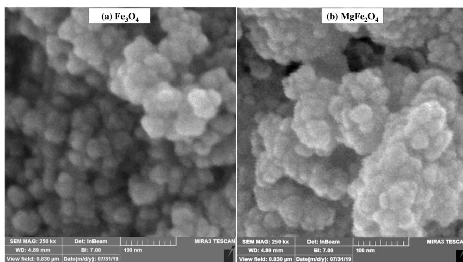
Figure 2. FESEM images of nano magnetic adsorbents: (a)  $\text{Fe}_3\text{O}_4$ , (b)  $\text{MgFe}_2\text{O}_4$ .
