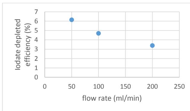
**Figure 2) Effect of the flow rate on photocatalytic output for hydrogen-producing reaction**
