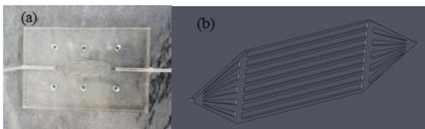
Figure 1) a) Image, b) schematic of optofluidic microreactor with rectangular micro-grooved
